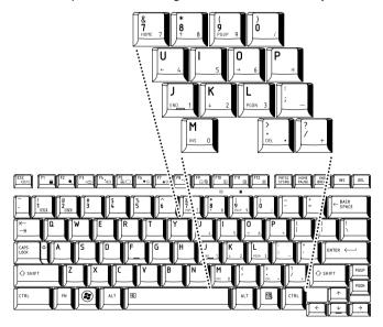
Figure 5-2 The numeric keypad overlay
